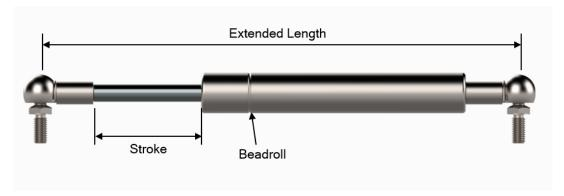
**Extended length** – The total length of the gas spring measured from the centre to centre of the end fits when the spring is fully extended.
